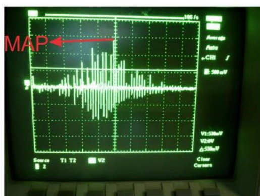
Figure 8 Sensor output when the handcuff starts to deflate 2
